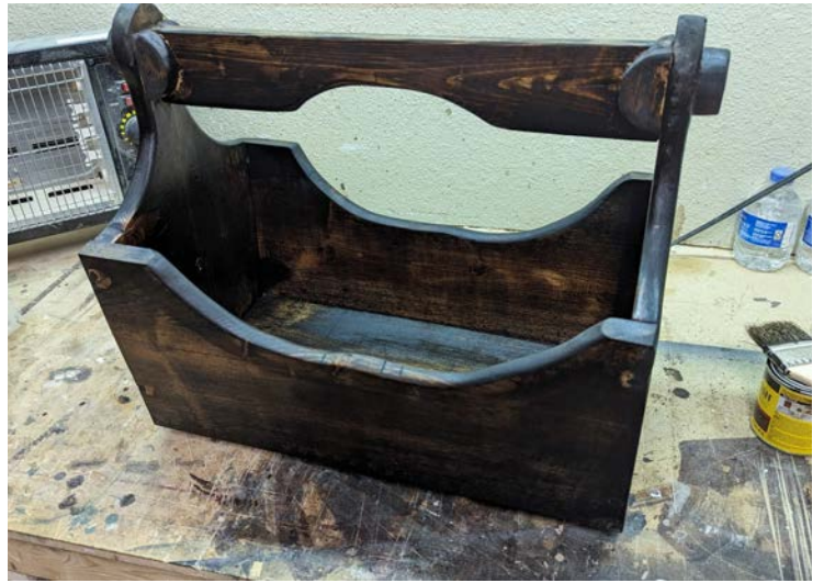
Wooden tote: Hand Tool only construction, with traditional woodworking tools and methods. The design is post period, but the joinery used is all documentable to pre-1600 tools and techniques. By HL Ivo Blackhawk.
